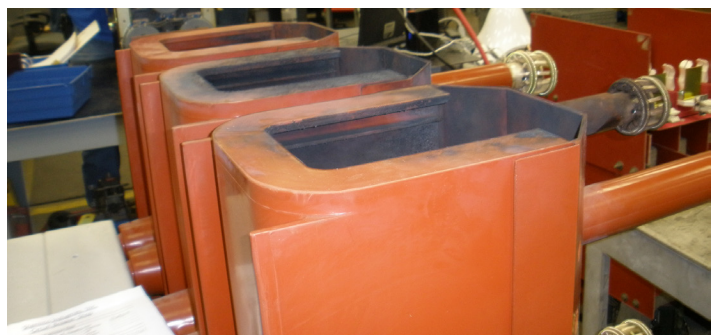
Photo 6. This image shows the aftermath of what happens when a vacuum bottle fails.
