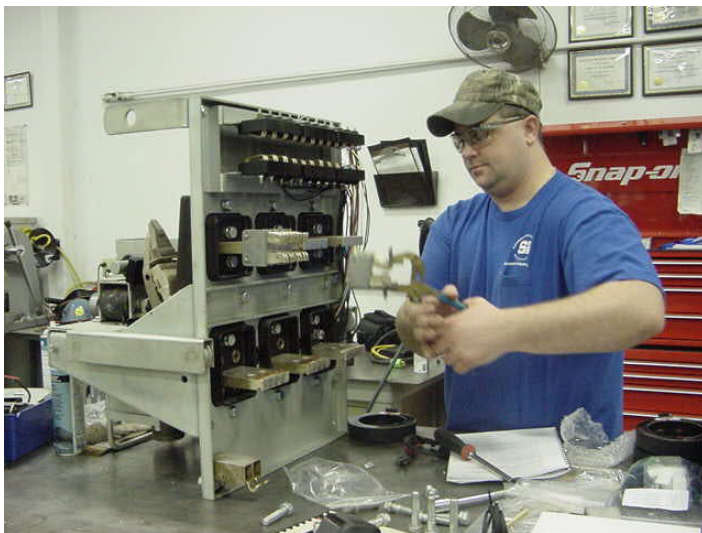
Photo 1. A technician working on a Westinghouse low-voltage power circuit breaker.
